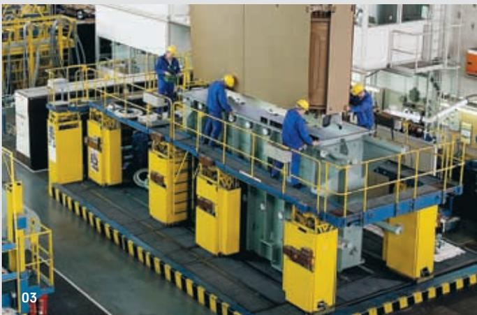
**01 Manual operation** | Siemens workers in Dresden carefully assemble the core of a transformer, layer by layer. The electrical steel they use to do so, which is produced by ThyssenKrupp Electrical Steel, is slit on special processing lines and punched into various shapes.
