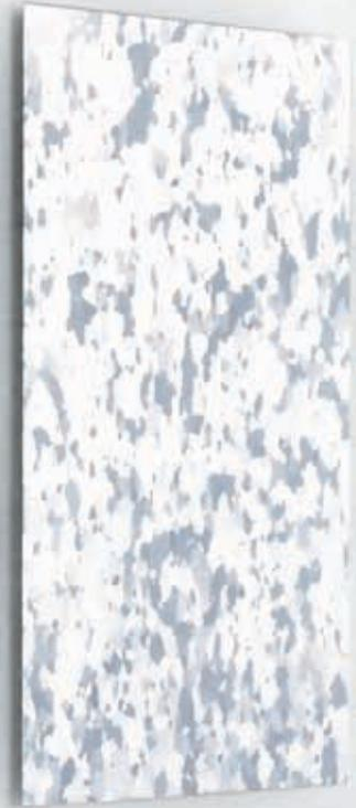
Typical grain structure of electrical steel
