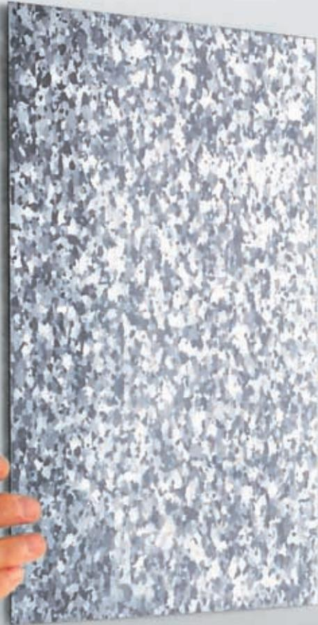
Typical grain structure of electrical steel
